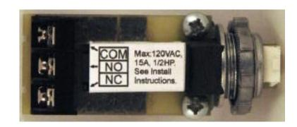
The Relay Module can be used to safely control (on/off) any 120V appliance using 12V signals. The Relay Module is just a simple SPDT relay that has been repackaged, having both Normally Closed (NC) and Normally Open (NO) contacts available through screw terminals. With the Common (COM) and NC contact, connected to a TV, Block Heater or Awning, it can be used as an Ignition Lock-out feature. Using the NO and COM contacts, the Relay module can control a Water Heater or Fireplace.
