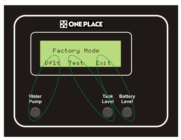
The **DNE PLACE MONITOR PANEL** has many safe guards to prevent improperly learning a feature. Should the Panel have learned something incorrectly, an option exists on the Panel to reset the original factory default, so that the Panel can re-learn the proper features.
