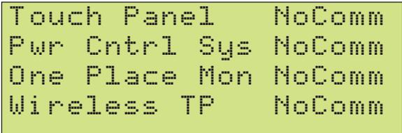
This screen simply shows if the PRECISION
