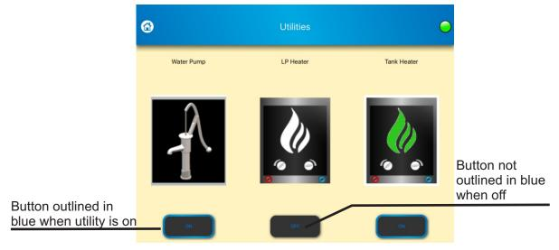
Utilities: This screen allows the user to turn on or off the water pump, liquid propane heater, and tank heater as necessary or as situations demand. Simply touch the button underneath the image to turn on or off. On the touch screen touching the on/off button or the image will operate the feature.
