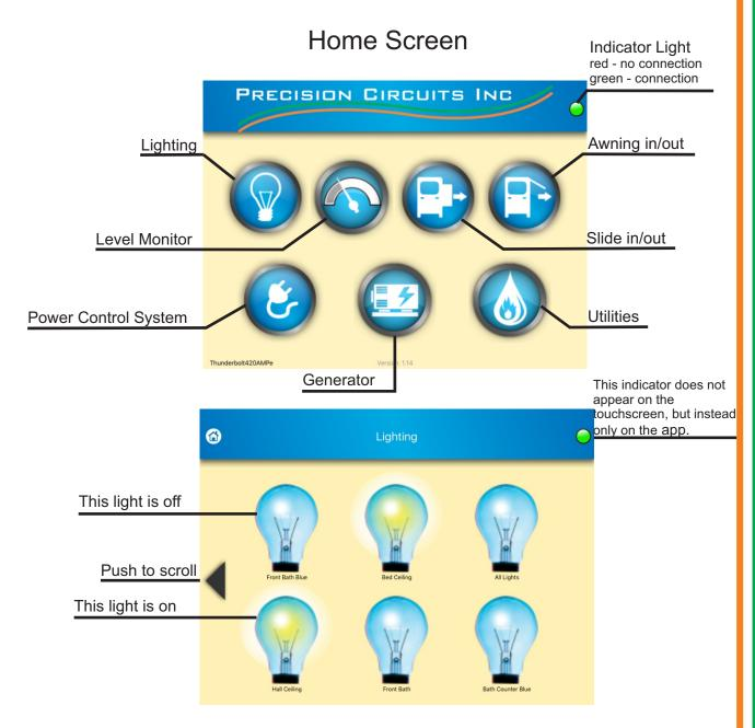
Lighting - Control every light in your RV from this screen. Use the arrow keys to scroll left and right to view each lighting option. In the image above, "Hall Ceiling" and "Bed Ceiling" indicate a light is on.
