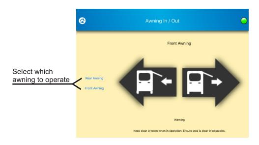
**Awning IN/OUT:** To move awning out, check the area surrounding your RV, and if there is enough room, push and hold the button on the right. Letting go of the button will stop the awning from moving. To bring the awning back in, push and hold the button on the left. If more than one person is trying to operate the awning via multiple devices, the person who was first in attempting operation will be the one able to carry out execution.
